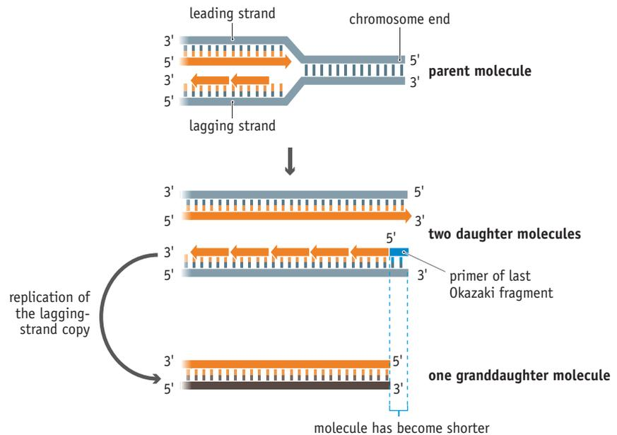
beyond the end of the lagging strand (Figure 11.19A). The absence of this Okazaki fragment means that the lagging-strand copy is shorter than it should be. If the copy remains this length, then when it acts as a parent polynucleotide in the next round of replication the resulting daughter molecule will be shorter than its grandparent.
