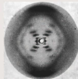
**FIGURE 4** Franklin's "photo 51" showing the diffraction pattern obtained with a fiber of DNA. The cross shape indicates that DNA has a helical structure, and the relative positions of the various dots and smears enable the periodicities within the molecule to be calculated. (From R. Franklin and R. G. Gosling, *Nature* 171: 740–741, 1953. With permission from Macmillan Publishers Ltd.)
