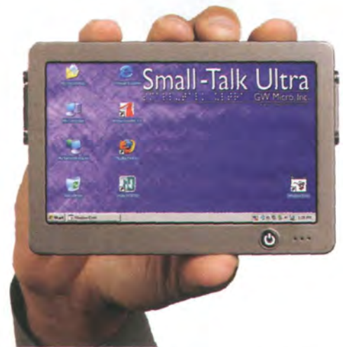
Small-Talk Ultra, a talking computer from GW Micro, which includes Window-Eyes – a screen reader for the blind
