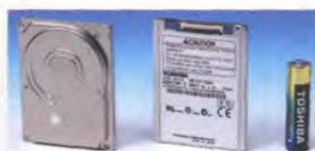
Toshiba's 1.8" hard drive; mini hard drives are used in small gadgets, such as PDAs and wristwatches
