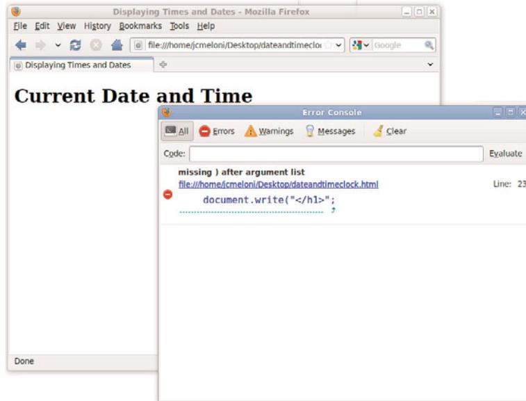
Although Internet Explorer displays error dialog boxes for each error, Firefox's JavaScript Console displays a single list of errors and enables you to test commands. For this reason, you might find it useful to install Firefox for debugging and testing JavaScript, even if Internet Explorer is your primary browser.
