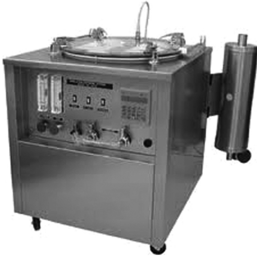
FIGURE 2.2 Glass-Col apparatus. This instrument is the advancement of earlier models developed by Middlebrook. Eighty to hundred mice can be exposed to aerosol at one time.
