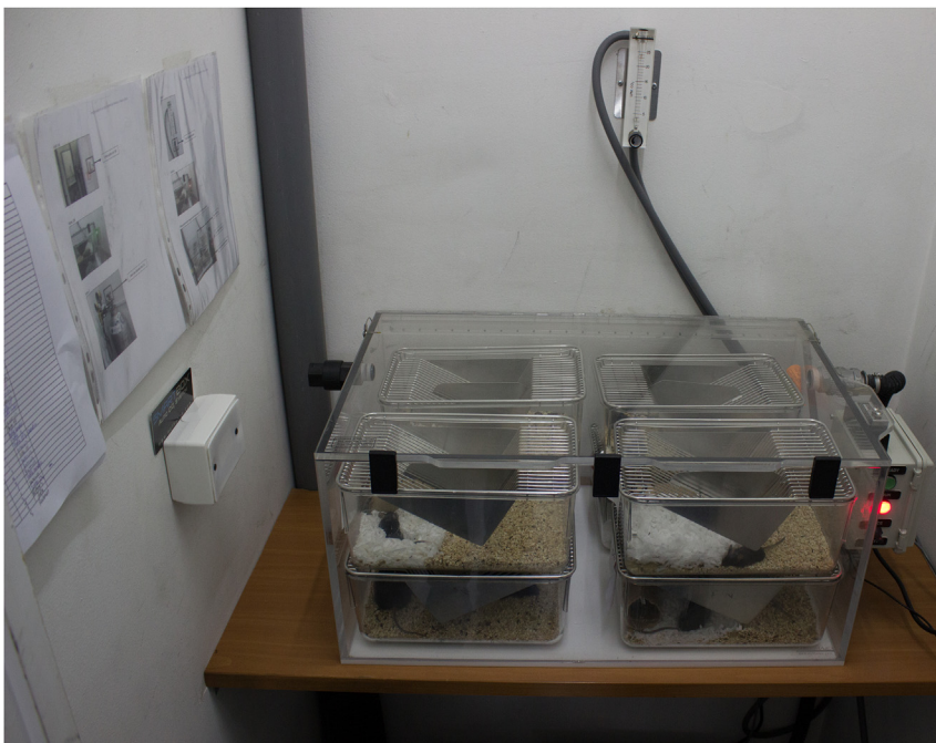
FIGURE 36.1 A carbon dioxide euthanasia chamber holding four cages of mice. When activated a light (right of figure) indicates gradual filling of the chamber with carbon dioxide and that the chamber is locked, preventing more animals to be added during the process. On the wall (back of the figure) is a flowmeter that closely regulates the rate at which carbon dioxide is added to the chamber. The system maintains an effective carbon dioxide concentration for a preset time and then automatically evacuates remaining carbon dioxide at the end of the cycle.
