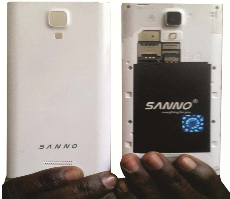
Figure 4.3b: Back cover screw holes
