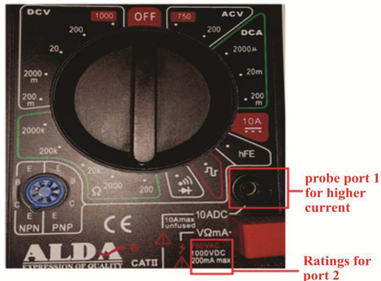
Figure 4.8: Digital Multimeter probe connection
