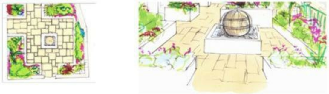
Random bond paving in 5 mixed sizes makes the area look wider and longer because of the mixed directions.
