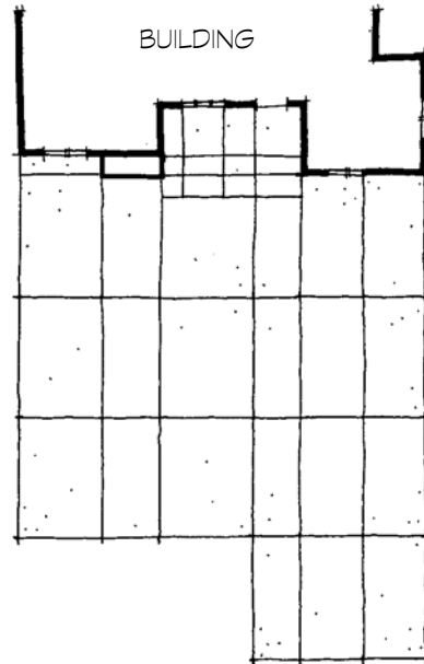
GRID BASED ON ADJOINING BUILDING
