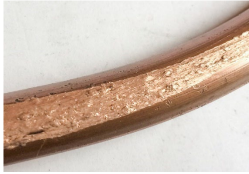
Fig. 10. The photo of the surface of the MF-100 contact wire after working in pair with the sample "Sample 4"
