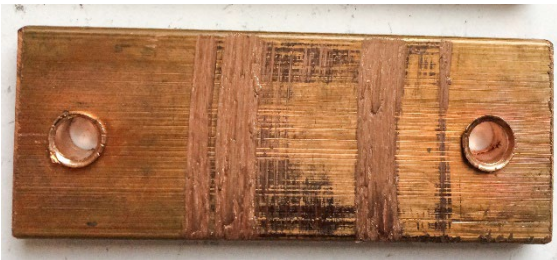
Fig. 9. The photo of "Sample 4" after jamming of the bench
