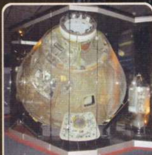
command module (CM): control centre & living quarters for crew
