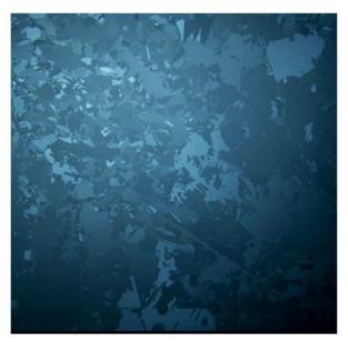
Multicrystalline Si with SiNx ARC and different grain size.
