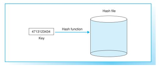
The idea behind hashing is to provide a function, the hash function, which is applied to the hash key of a record and yields the address of the file record. If the file records are numerated and if the hash key equals the record number, a simple hash function can be the identical function. However, hash keys, such as account or insurance numbers, consist of a fixed number of digits that do not start with 0.
