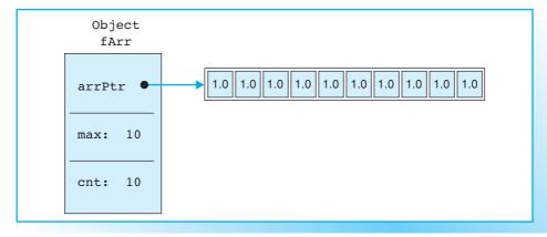
The memory for the array elements is not contained in a FloatArr object and must be allocated dynamically by the constructor. The object itself only occupies the memory required for the data members arrPtr, max, and cnt. Thus, sizeof (FloatArr) is a constant value that defaults to 12 bytes for 32 bit computers.
