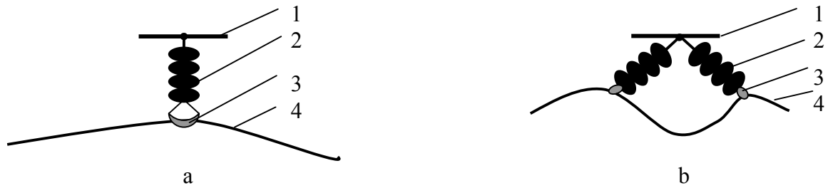
Fig. 1.14. The wire fastened in phase on the intermediate (a) and anchor (b) support: 1 – crossarm; 2 – insulator string; 3 – terminal; 4 – wire
