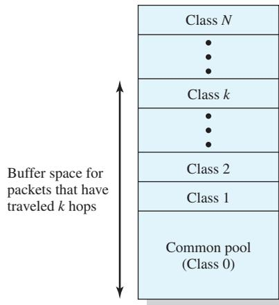
**Figure 18.18** Structured Buffer Pool for Deadlock Prevention
