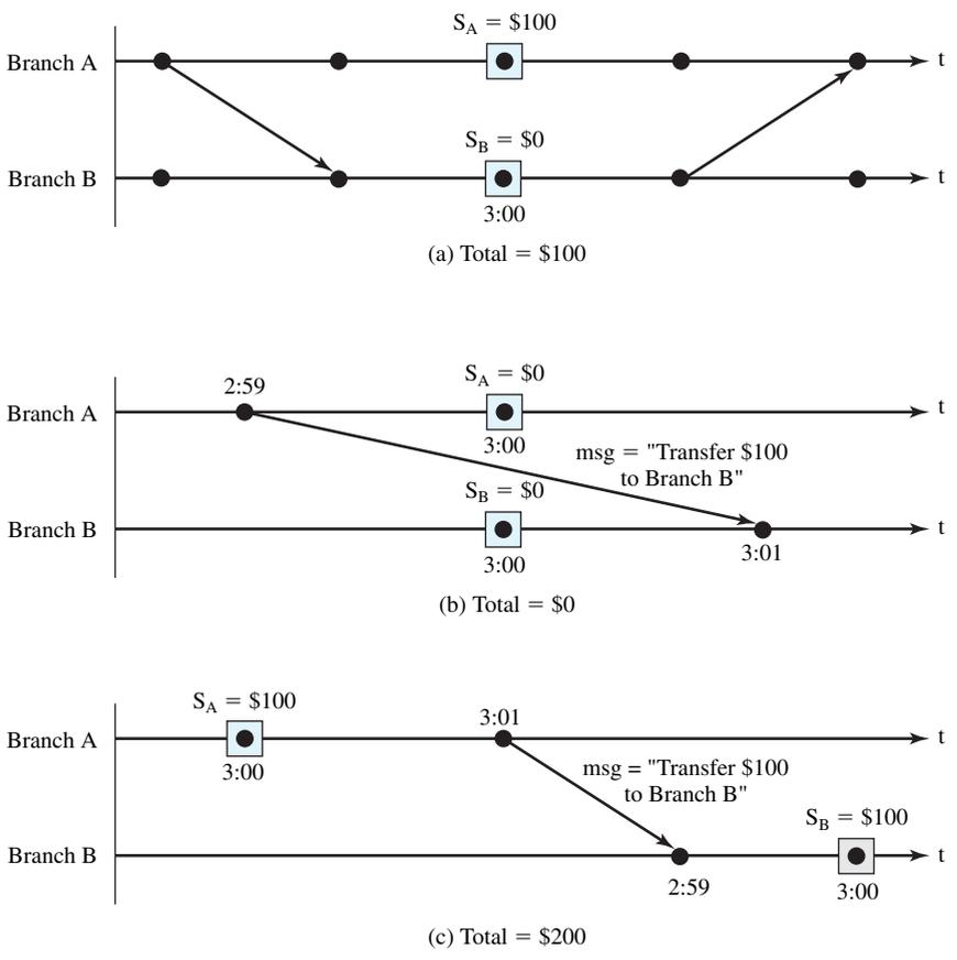
**Figure 18.3** Example of Determining Global States
