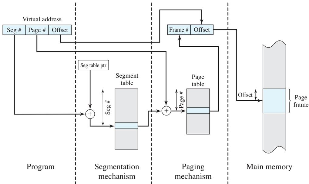
**Figure 8.13** Address Translation in a Segmentation/Paging System
