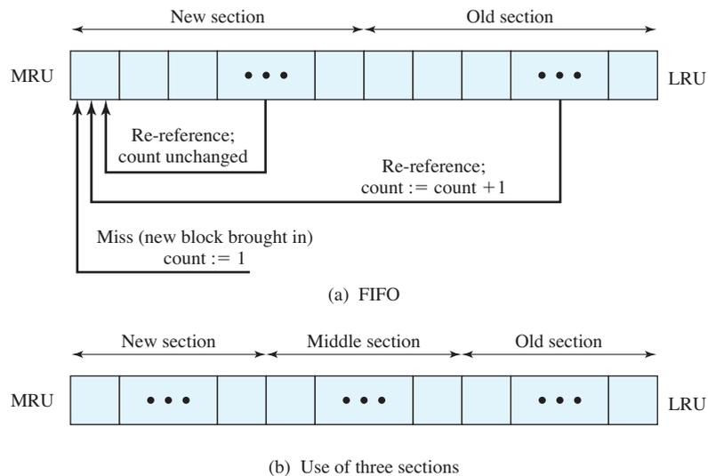
**Figure 11.9** Frequency-Based Replacement
