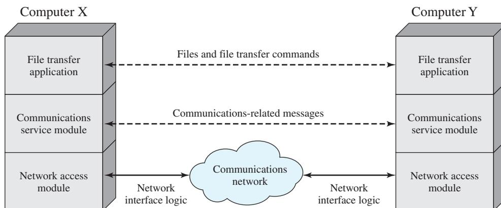
**Figure 17.1** A Simplified Architecture for File Transfer
