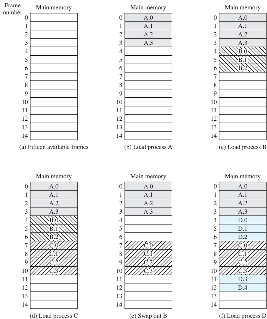
**Figure 7.9** Assignment of Process to Free Frames
