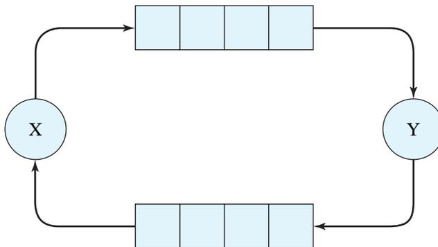
**Figure 18.19** Communication Deadlock in a Distributed System
