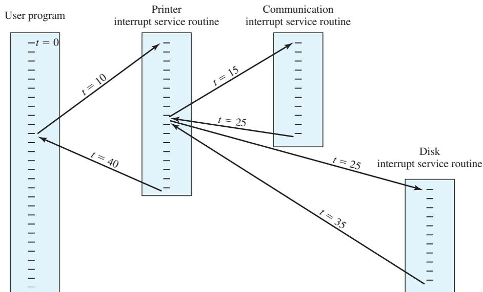
**Figure 1.13** Example Time Sequence of Multiple Interrupts
