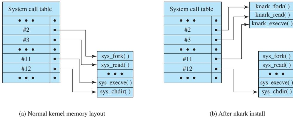
**Figure 14.6** System Call Table Modification by Rootkit
