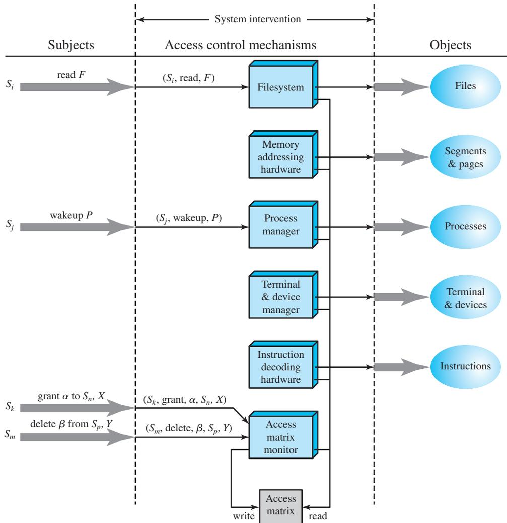
**Figure 15.5** An Organization of the Access Control Function
