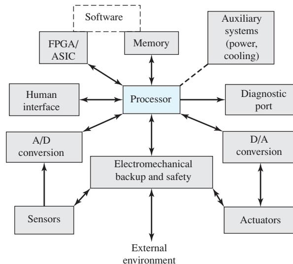
**Figure 13.1** Possible Organization of an Embedded System
