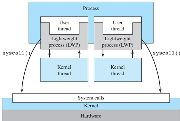
**Figure 4.15 Processes and Threads in Solaris [MCDO07]**
