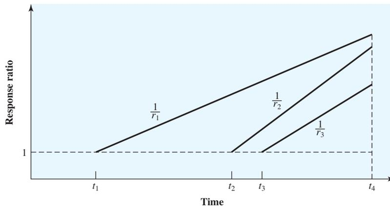
Figure 9.18 Response Ratio as a Function of Time
