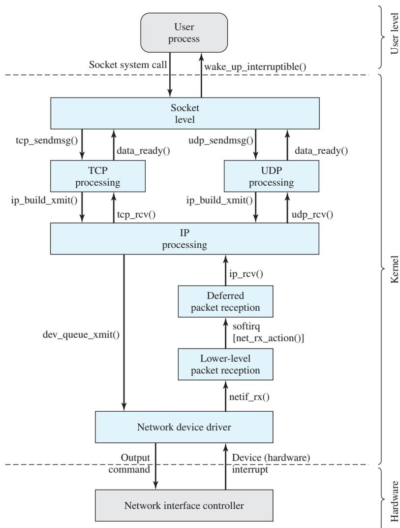
**Figure 17.7** Linux Kernel Components for TCP/IP Processing
