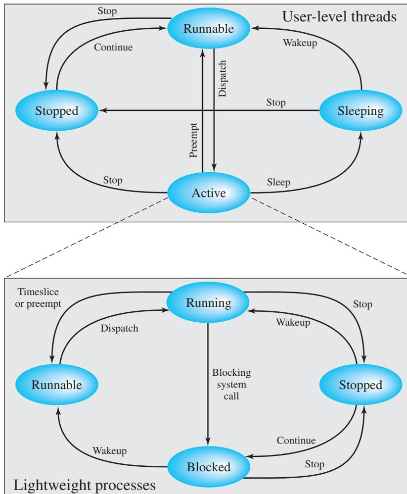
**Figure 4.19** Solaris User-Level Thread and LWP States
