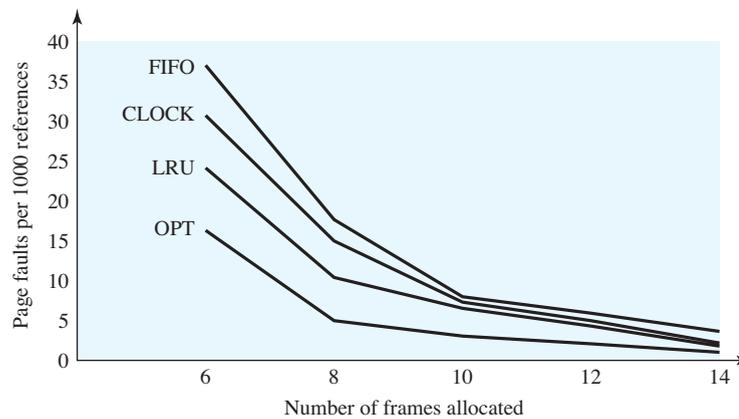
**Figure 8.17** Comparison of Fixed-Allocation, Local Page Replacement Algorithms
