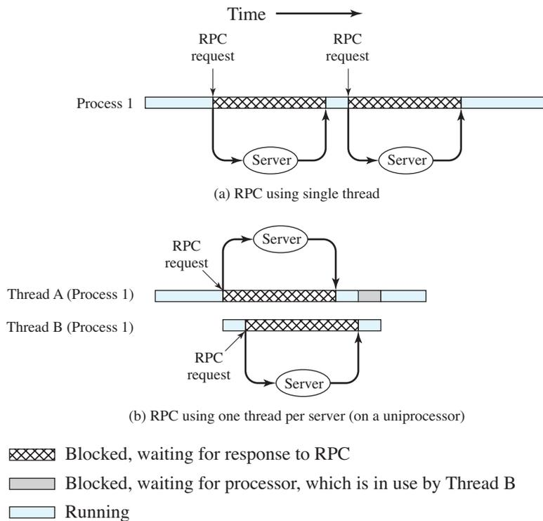
**Figure 4.3** Remote Procedure Call (RPC) Using Threads
