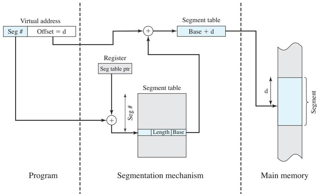
**Figure 8.12** Address Translation in a Segmentation System
