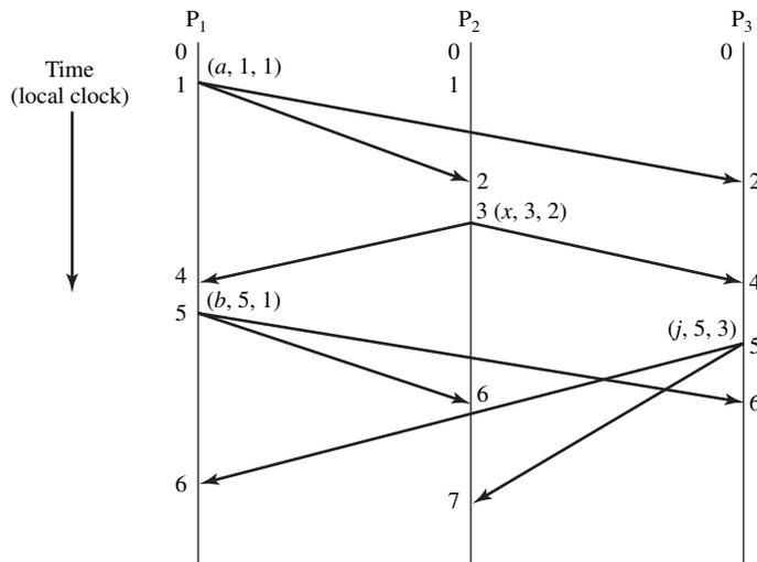
**Figure 18.8** Example of Operation of Timestamping Algorithm
