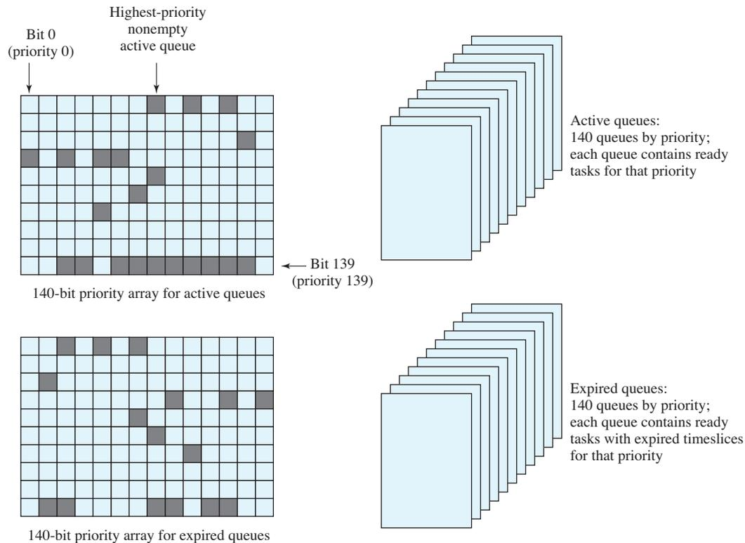
**Figure 10.12** Linux Scheduling Data Structures for Each Processor
