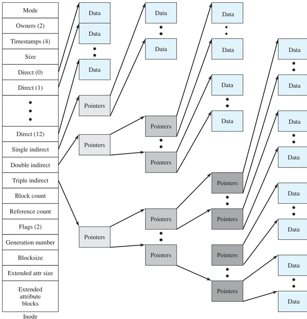
**Figure 12.14** Structure of FreeBSD inode and File
