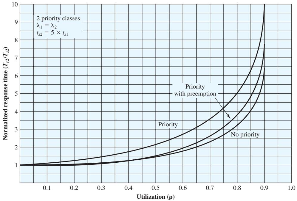
Figure 9.13 Normalized Response Time for Longer Processes
