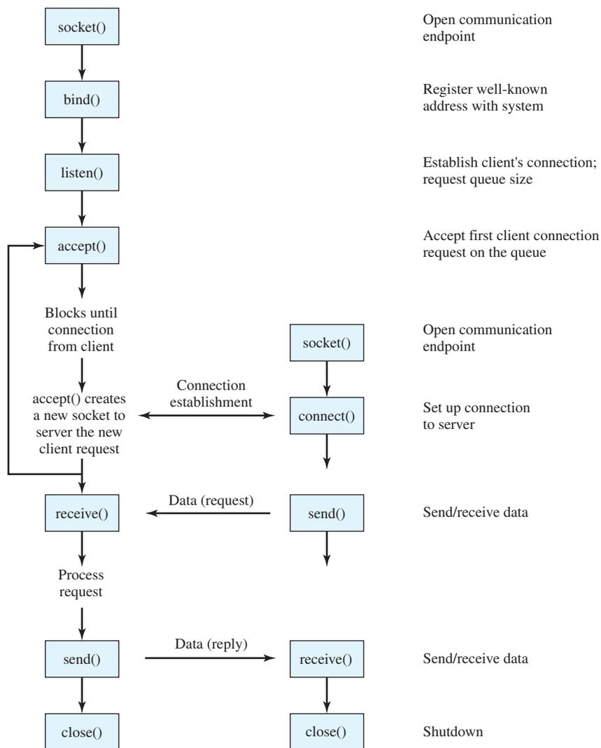
**Figure 17.6** Socket System Calls for Connection-Oriented Protocol
