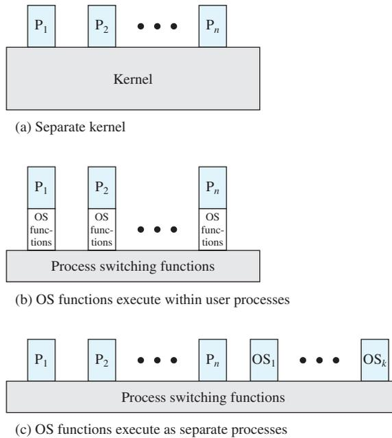
**Figure 3.15** Relationship between Operating System and User Processes
