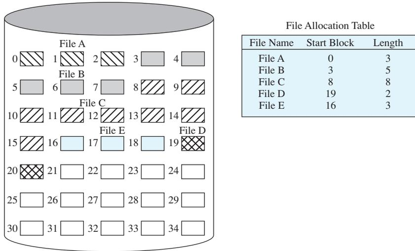
**Figure 12.8** Contiguous File Allocation (After Compaction)
