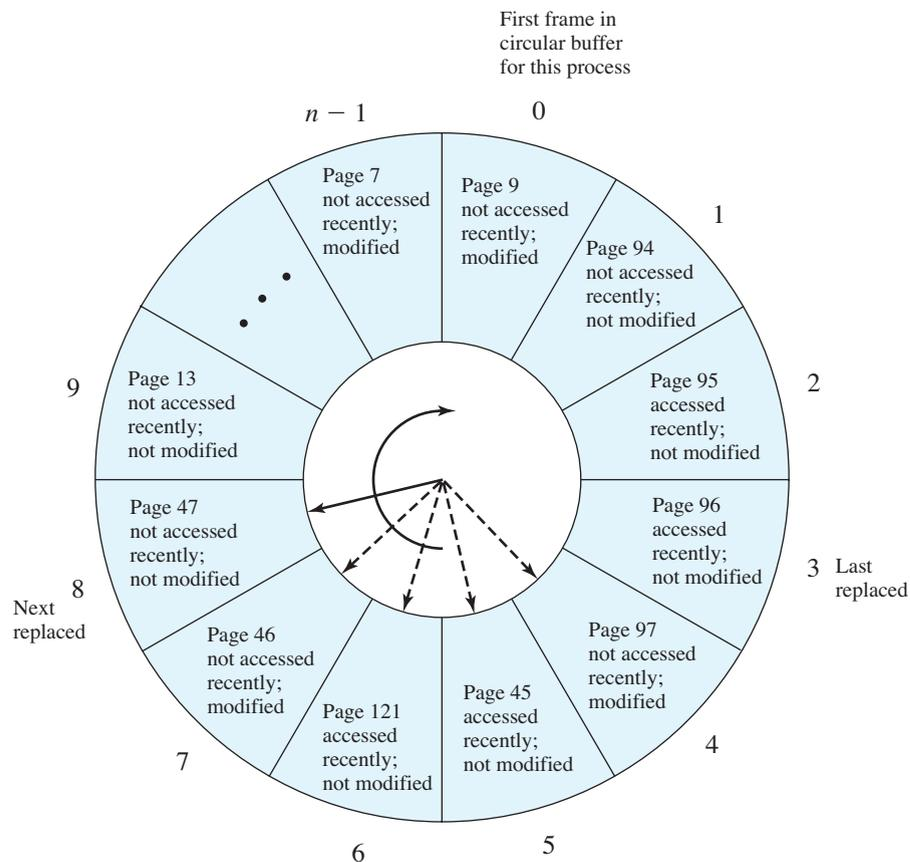
**Figure 8.18** The Clock Page Replacement Algorithm [GOLD89]
