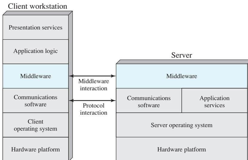
**Figure 16.8** The Role of Middleware in Client/Server Architecture
