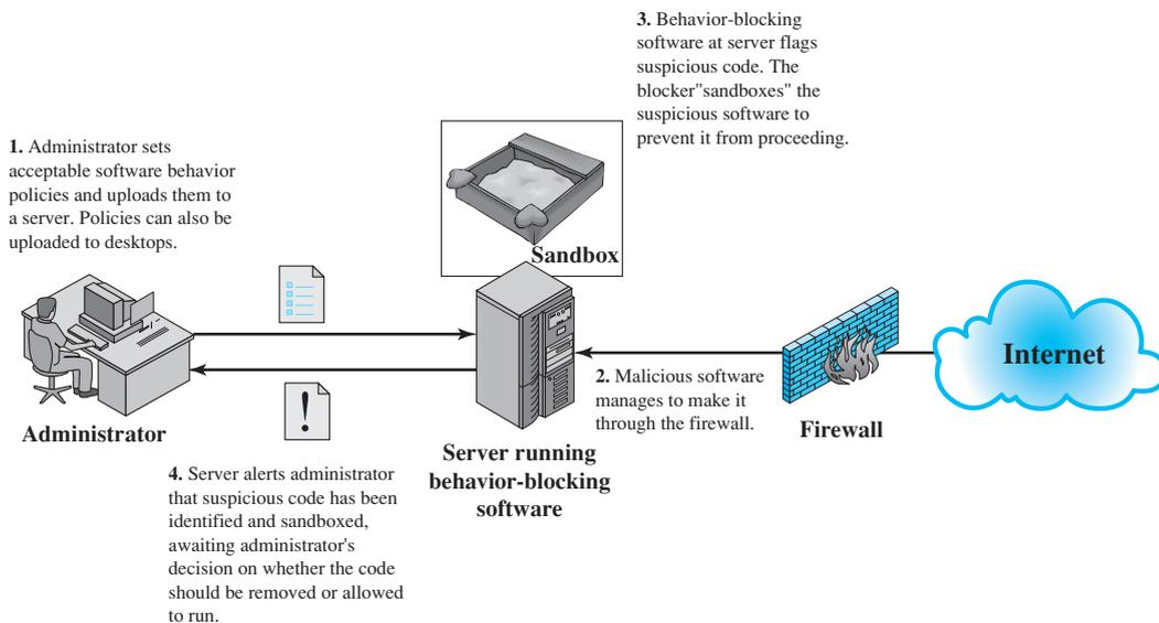
**Figure 15.10 Behavior-Blocking Software Operation**
