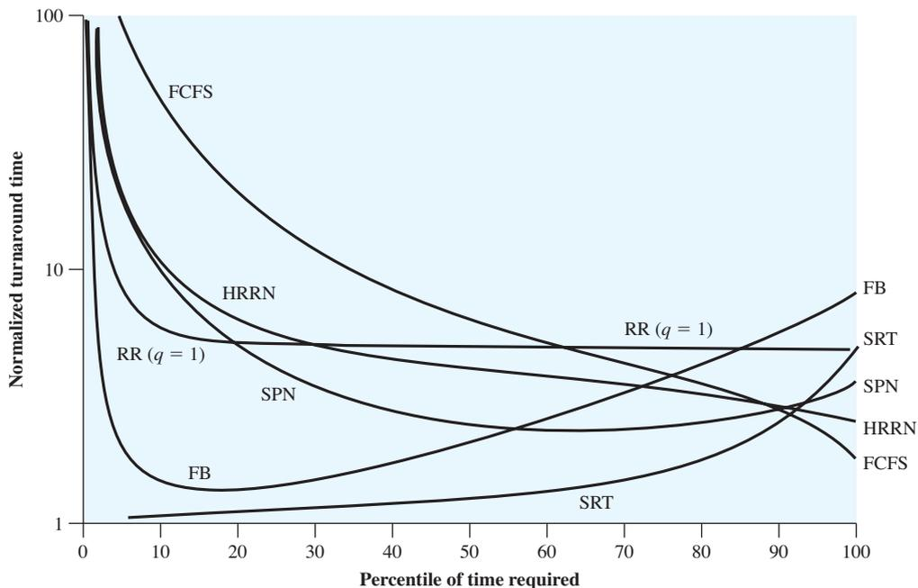
**Figure 9.14** Simulation Result for Normalized Turnaround Time
