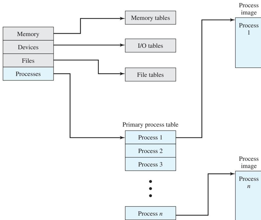
**Figure 3.11** General Structure of Operating System Control Tables
