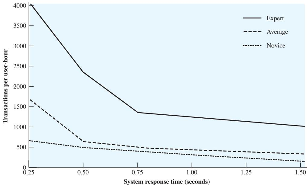
**Figure 9.20** Response Time Results for High-Function Graphics
