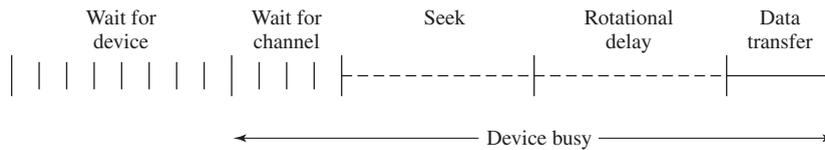
**Figure 11.6** Timing of a Disk I/O Transfer
