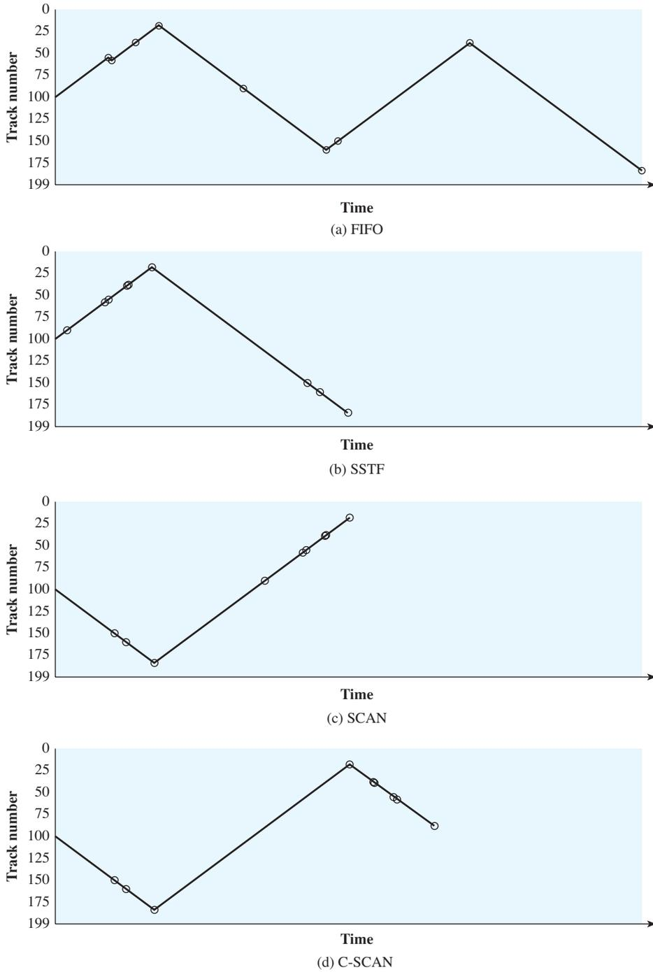
**Figure 11.7** Comparison of Disk Scheduling Algorithms (see Table 11.3)
