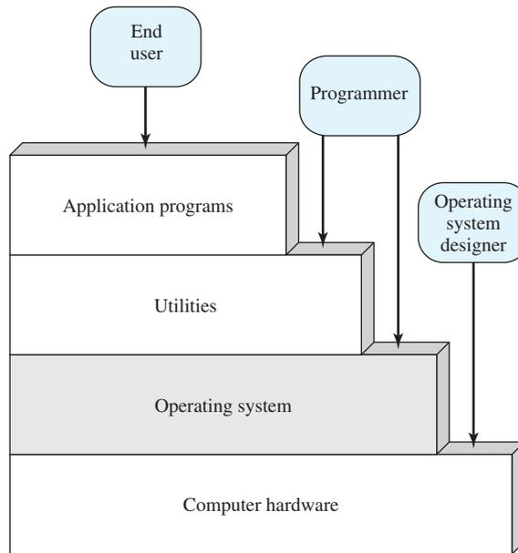
**Figure 2.1** Layers and Views of a Computer System
