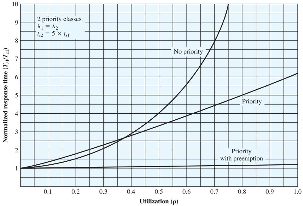
Figure 9.12 Normalized Response Time for Shorter Processes
