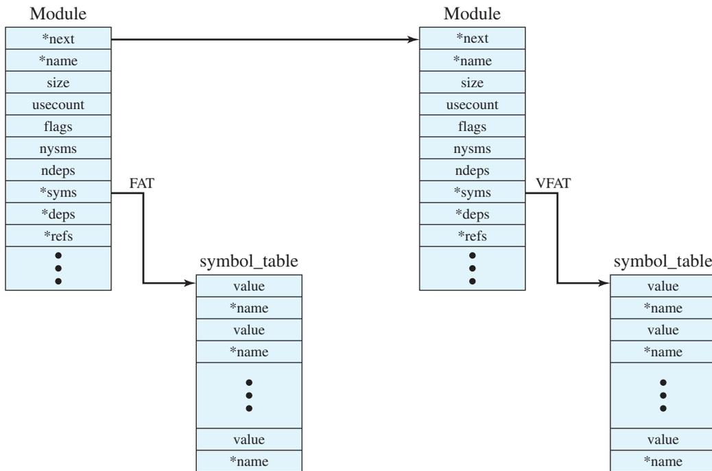
**Figure 2.17** Example List of Linux Kernel Modules
