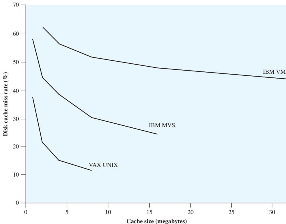
**Figure 11.11** Disk Cache Performance Using Frequency-Based Replacement
