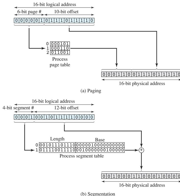
**Figure 7.12** Examples of Logical-to Physical Address Translation
