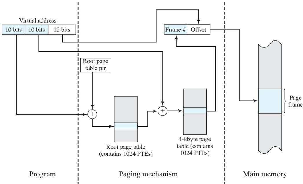
Figure 8.5 Address Translation in a Two-Level Paging System
