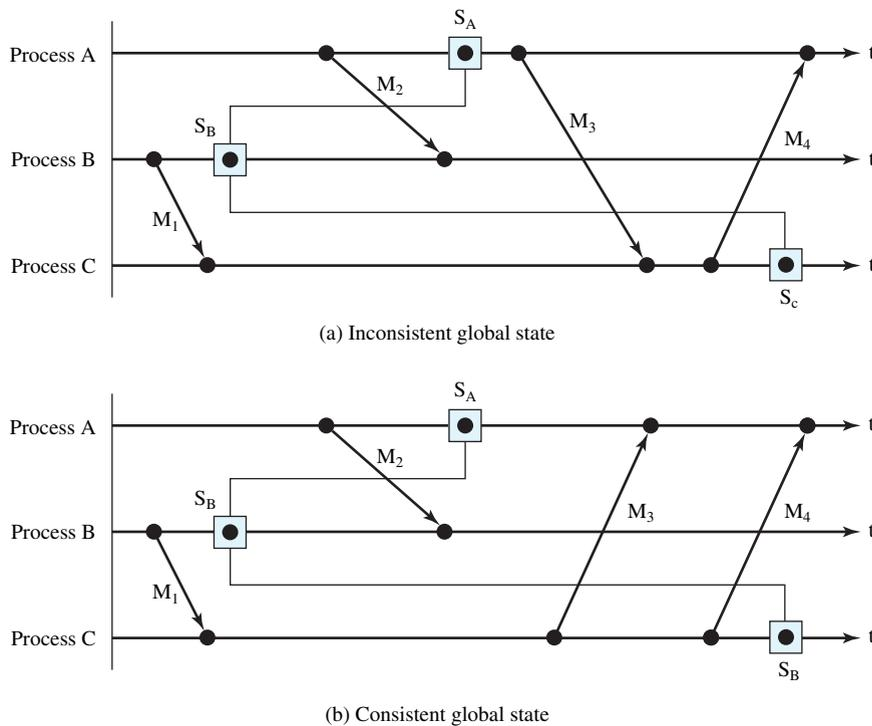
**Figure 18.4** Inconsistent and Consistent Global States
