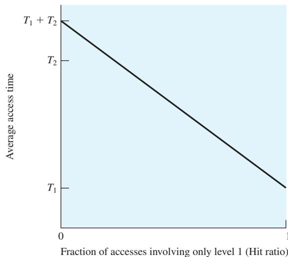
**Figure 1.15** Performance of a Simple Two-Level Memory
