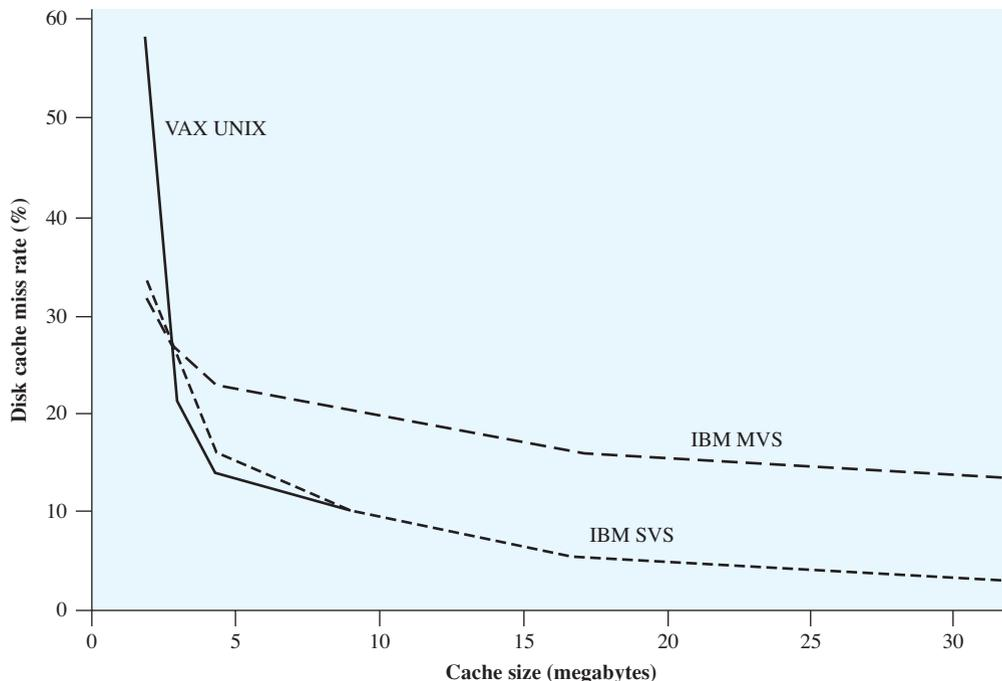
**Figure 11.10** Some Disk Cache Performance Results Using LRU
