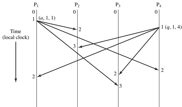
**Figure 18.9** Another Example of Operation of Timestamping Algorithm
