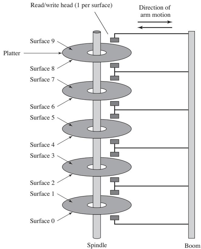
**Figure 11.18** Components of a Disk Drive
