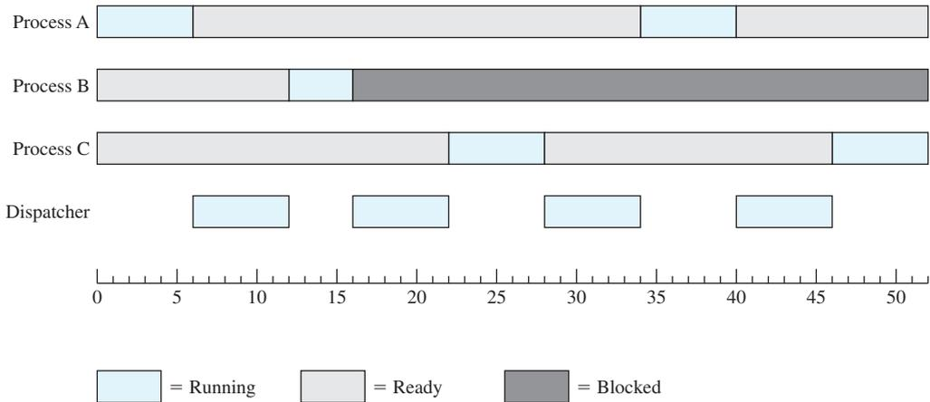
Figure 3.7 Process States for the Trace of Figure 3.4
