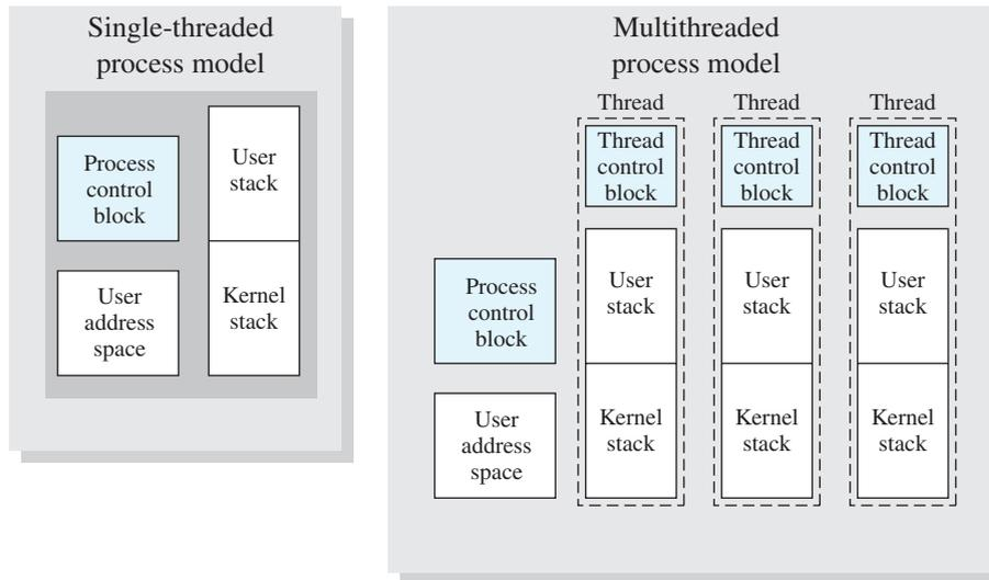
**Figure 4.2** Single Threaded and Multithreaded Process Models
