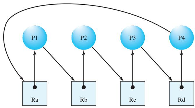
Figure 6.6 Resource Allocation Graph for Figure 6.1b
