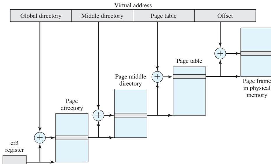
**Figure 8.25** Address Translation in Linux Virtual Memory Scheme
