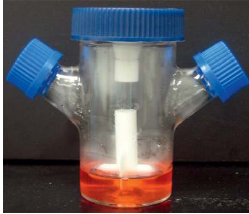
FIGURE 17.10 A spinner flask, an example of a dynamic culture bioreactor. Photo courtesy of Prof. Taby Ahsan, Tulane University.
