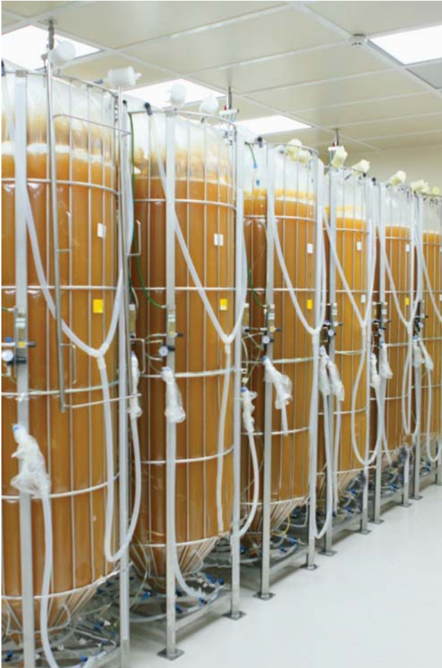
Figure 10.4 Disposable pneumatic bioreactors that lie at the center of the ProCellEx ® platform. Structures assembled around each reactor provide structural integrity, allowing for cultivation at 400-l volumes [7].
