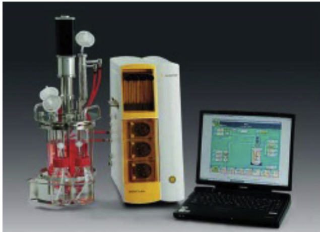
Figure 2.2 A commercial laboratory reactor (Biostat® A plus from Sartorius) for medium volume between 0.4 and 5 l. The reactor is supported by packages for either microbial cell or animal/plant cell cultures. The microbial package includes two 6-blade Rushton
