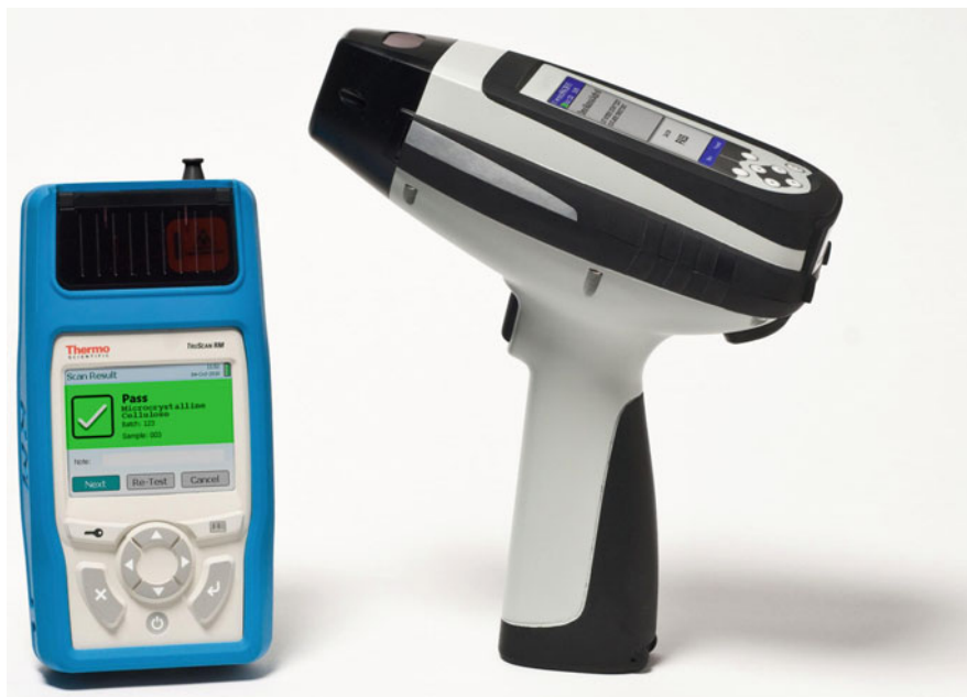
Fig. 2 Handheld NIR material analyzer (Thermo Fisher microPHAZIR RX, http://www.thermoscientific.com )
