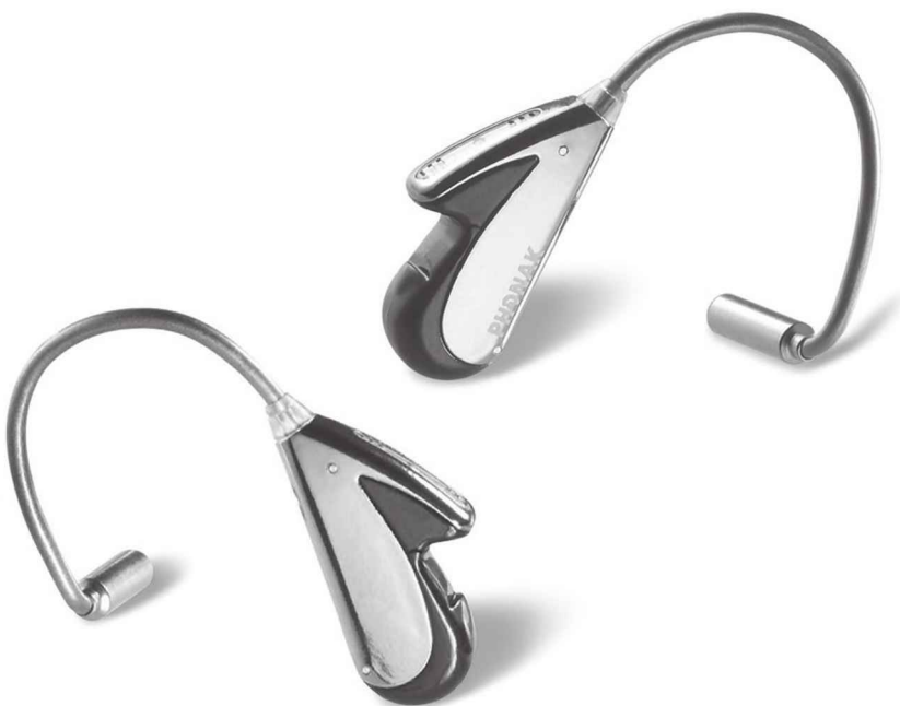
Figure 12-1. The iSense, a miniaturized FM receiver, was designed for listeners with normal hearing sensitivity and can be used with a variety of FM transmitters. Photo Courtesy of Phonak.
