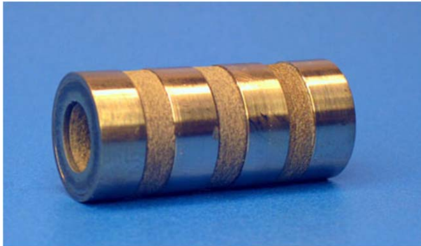
Figure 21. Tubular TEG consists of four p-type n-type thermoelements PbTe (from reference [37])
