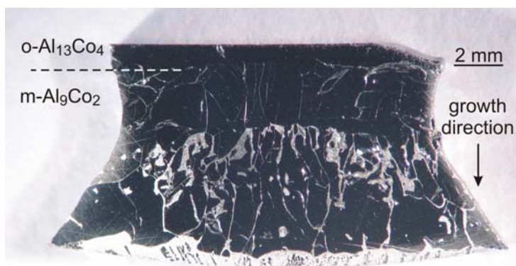
Fig. 7 Longitudinal section through the very rare part of an \text{Al}_{13}\text{Co}_4 single crystal grown parallel to [001] from an Al-rich solution of initial composition \text{Al}_{86.5}\text{Co}_{13.5} . With the growth temperature at the phase boundary falling below the peritectic temperature of 974^\circ\text{C} , polycrystalline growth of monoclinic \text{Al}_9\text{Co}_2 onto the orthorhombic \text{Al}_{13}\text{Co}_4 single crystal occurred resulting in stress-induced cracks. Bright spots are eutectic structures of practically pure Al resulting from fast cooling down at the end of the experiment.
