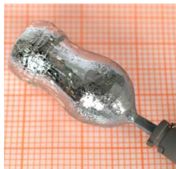
Fig. 6 \text{Al}_{13}\text{Fe}_4 single crystal grown by the Czochralski method from an Al-rich solution of initial composition \text{Al}_{89.5}\text{Fe}_{10.5} using a [010] oriented single-crystalline native seed.
