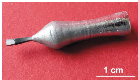
Fig. 5 \text{Al}_{13}\text{Co}_4 single crystal grown by the Czochralski method from an Al-rich solution of initial composition \text{Al}_{86.5}\text{Co}_{13.5} using a [001] oriented single-crystalline native seed. (Online color for figures 5 and 6 at www.crt-journal.org )
