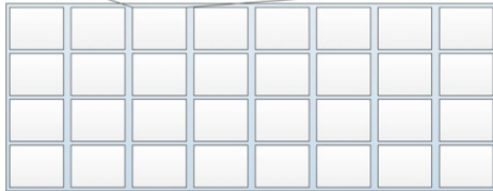
AMD Radeon HD7970 32 cores 1 scalar unit and 4 16-wide SIMD units per core 4-8 set of 64-wide vector registers per SIMD unit, 16-32 per core
