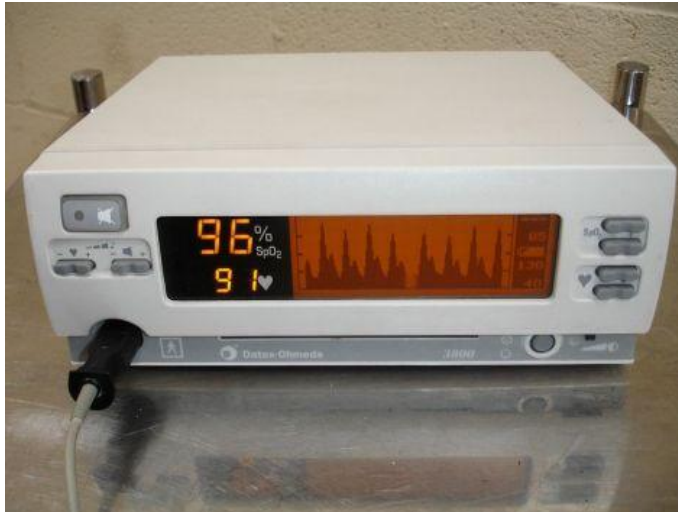
Figure 12: Pulse oximeter displaying oxygen saturation (SpO 2 ) in the blood and the pulse rate
