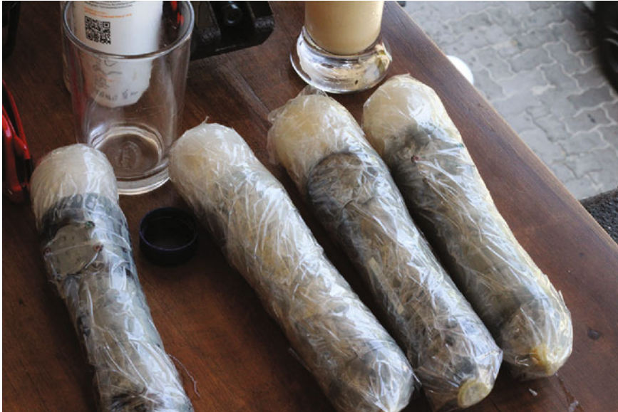
Fig. 12 PlayStation Move controllers waterproofed with condoms and sticky tape. Image credit Ida Marie Toft
