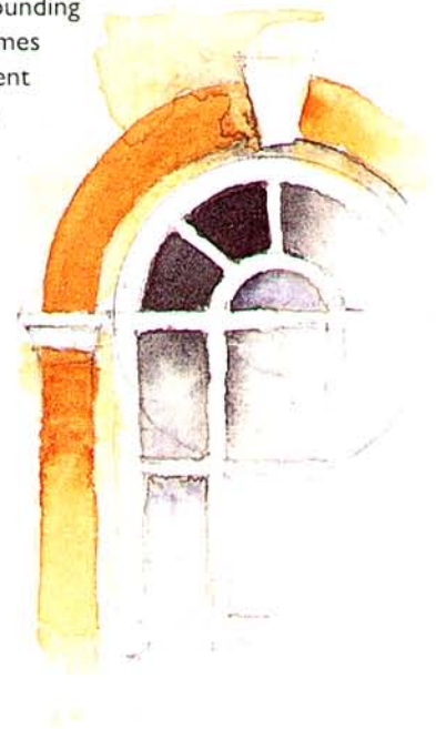
The centre of this window crossbar is the centre of the circle on which the window frame is built
