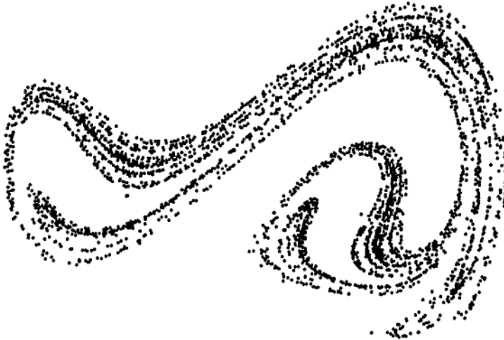
Figure 9-8 (c) Fractal structure of the Poincaré map of a mass in a two-well potential (see Moon, 1992).
