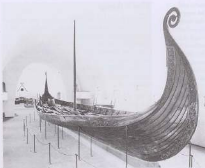
The Oseberg Viking ship, made in about AD 800, was 21 metres long and carried about 35 men. Although this particular ship was probably only used along the coast, ships of similar size were used to invade Britain. Their design was brilliant. When an exact copy of similar ship was used to cross the Atlantic to America in 1893, its captain wrote, "the finest merchant ships of our day . . . have practically the same type of bottom as the Viking ships."
