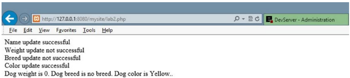
Figure 4-3. Output with invalid weight (1000) and invalid breed ('Lab12') in Dog class— dog.php and lab.php
