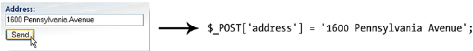
Figure 3-4. You can retrieve the values of user input through the $_POST array, which is created automatically when a form is submitted using the post method
