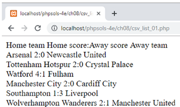
Figure 8-12. The generator processes every line of the CSV file, including the column titles
