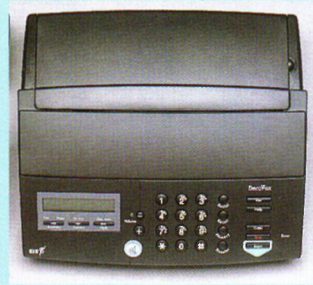
A fax machine sends and receives copies of original documents via a phone line
