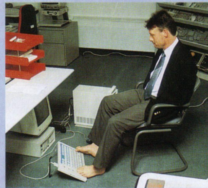
Bob Love was born with no arms. He uses an overlay keyboard with his feet and the computer and monitor on the floor. The key overlays give a much larger surface for each key.
