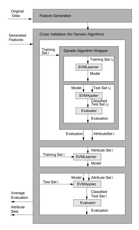
Figure 1.1: Nested operator chain for feature selection using a genetic algorithm.
