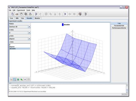
Figure 1.3: RAPIDMINER screenshot of the continuous result display of a parameter optimization process.
