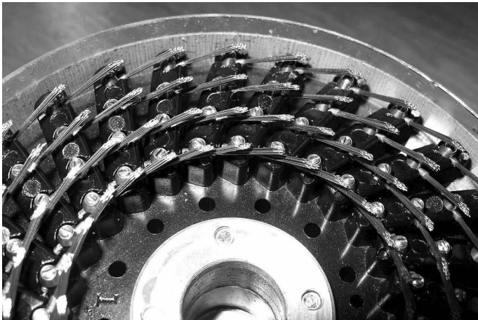
Figure 5.4 Back of a drum showing wire brushes.
