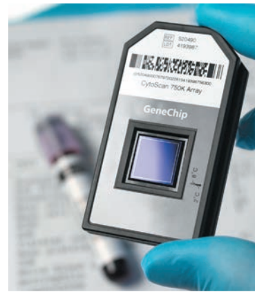
FIGURE 21.15 A commercially available DNA microarray, called a GeneChip®, marketed by Affymetrix, Inc. This particular microarray can be used to analyze expression for approximately 50,000 RNA transcripts. It contains 22 different probes for each transcript and allows scientists to simultaneously assess the expression levels of most of the genes in the human genome.
