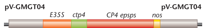
FIGURE ST 4.5 Portion of plasmid pV-GMGT04 used to create Roundup-Ready soybeans. A 1365-bp fragment encoding the EPSPS enzyme from Agrobacterium CP4 was cloned downstream from the cauliflower mosaic virus E35S promoter and the petunia chloroplast transit peptide signal sequence ( ctp4 ). CTP4 signal sequences direct the EPSPS protein into chloroplasts, where aromatic amino acids are synthesized. The CP4 epsps coding region was cloned upstream of the nopaline synthase ( nos ) transcription termination and polyadenylation sequences. The CP4 epsps sequences encode a 455-amino-acid 46-kDa ESPSP protein.
