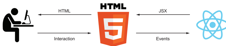
Figure 8.1 Information flow between React and the user goes through the HTML. Imagine the user visiting a login page. The user inputs the email and password, the browser forwards those interactions as events to React, the application then generates the JSX required to display a green checkmark next to each input as it's filled, and the browser renders the corresponding HTML to display to the user.
