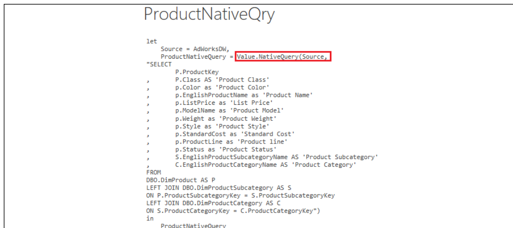
Figure 2.18: The Value.Native function used to pass a SQL statement to a source system
