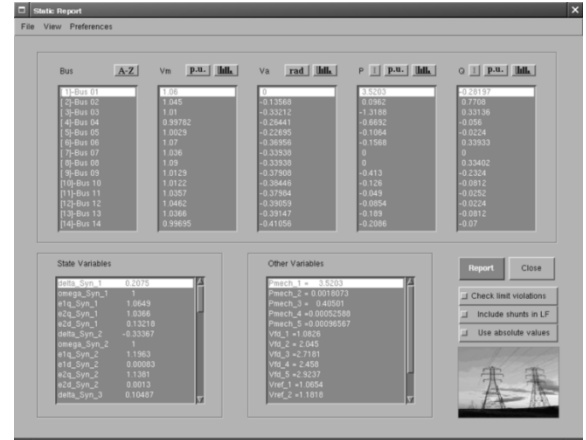
Fig. 6. GUI for power flow reports. The results refer to the IEEE 14-bus test system.
